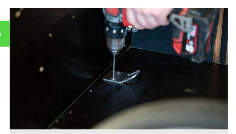
Mount your brackets and back plate with the stainless steel bolts, washers and nuts
